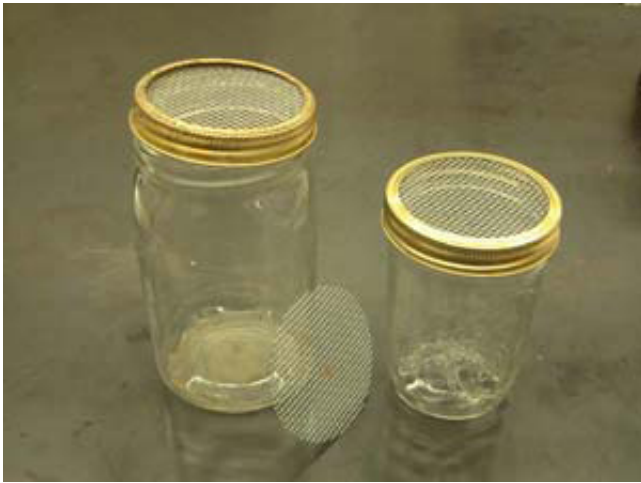
A wide-mouth canning jar with a cover made of 8x8 hardware cloth
